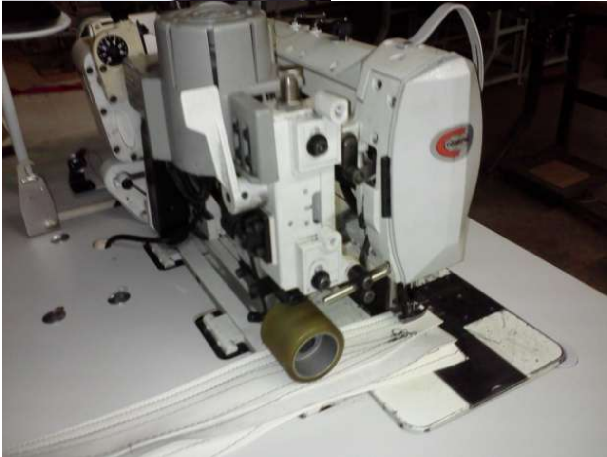
CONSEW 339RB WITH TOP AND BOTTOM DRIVE PULLER NEW LARGE TABLE TOP
